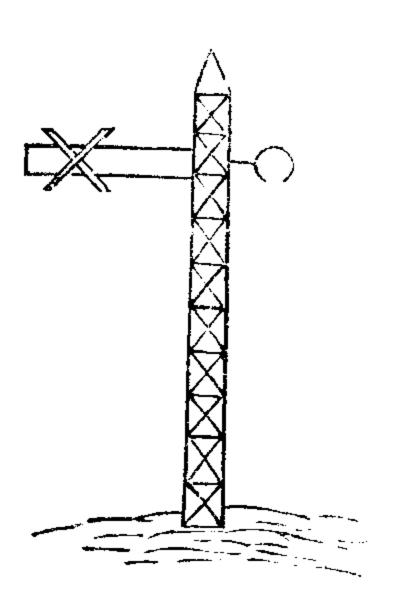
9.—Fixed signals shall be fixed on the side of the line on which they can be seen by Drivers of approaching trains, but the left hand side of the track is to be preferred unless the sighting is greatly interfered with.
