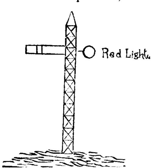
and by night, by showing a red light. When the Semaphore arm is so raised or a red light is shown, the signal is said to be "on," and signifies "Stop Dead," do not pass until the arm is lowered, or at night till the light is changed to green.
