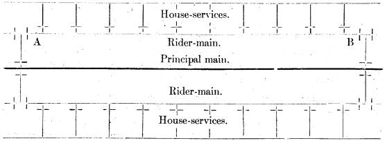
The house-services should be disconnected from the principal main, and connected to the rider-mains. In this way, the Town would be divided into blocks
